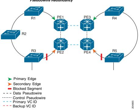
Figure D-6 Pseudowire Connectivity, Dual-Homed N-PEs on Both Sides of the Network, with No Pseudowire Redundancy
